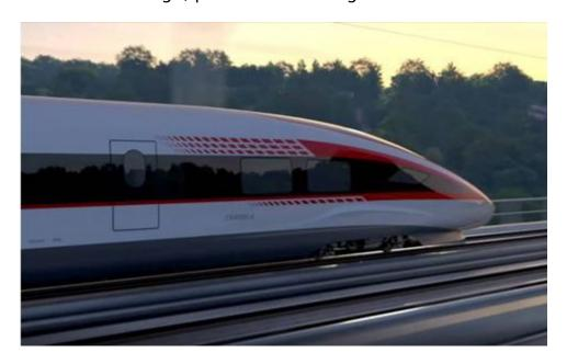
The train has been developed for cross-border operation between China's 1 435 mm gauge network and the 1 520 mm gauge used in neighbouring Russia and the CIS countries. The manufacturers cite one potential application as a Beijing – Moscow through service. A multi-system traction package will allow the train to run on different power supplies.
