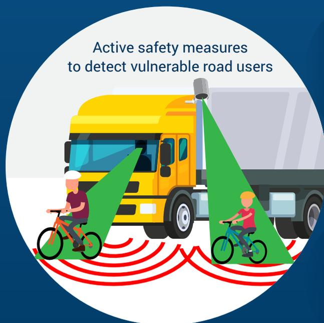
Moreover, contrary to 'direct vision' low-entry cabs, **active safety measures will actively draw the attention of the driver to the critical area or the VRUs concerned**. Even with the widest possible field of view in a low-entry cabin, a truck driver can only look in one direction at a time and still might fail to notice a pedestrian or cyclist on the other side of the vehicle.
